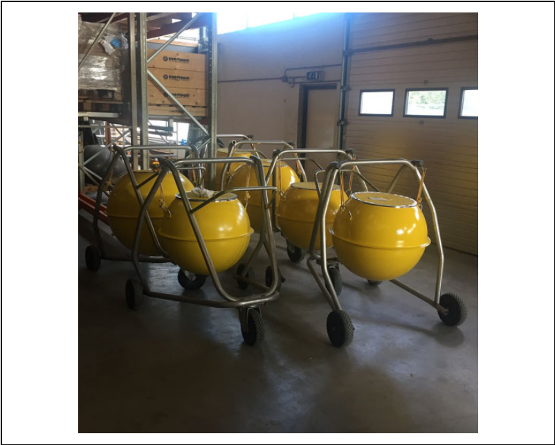
Figure 5. Datawell Waveriders on the factory floor, ready to be shipped. Photo by author.
