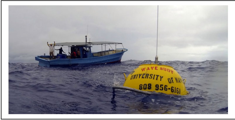
Figure 1. Datawell Directional Waverider buoy moored off Majuro Atoll in the Republic of the Marshall Islands as part of the Pacific Islands Ocean Observing System. Photo by Greg Zegas. http://www.hawaii.edu/news/2014/07/10/wave-buoy-in-majuro-helps-keep-islanders-safe/ .
