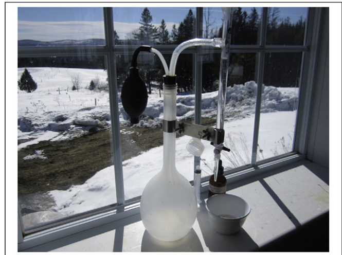
Figure 4. An acidity titrator in the cheeseroom of Jasper Hill Farm, Greensboro, Vermont. Photo by author.
