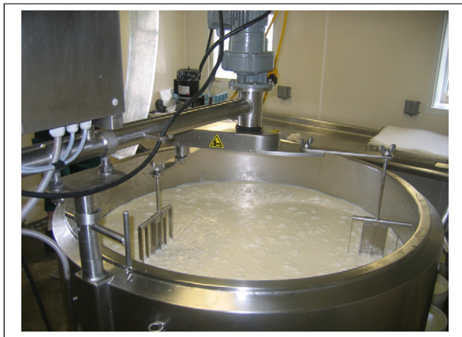
Figure 2. Mechanical stirring arm affixed to a 130-gallon vat. Photo by author.
